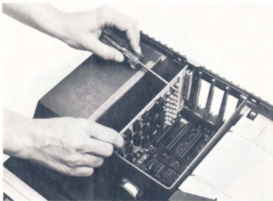
Removing a Peripheral Card
