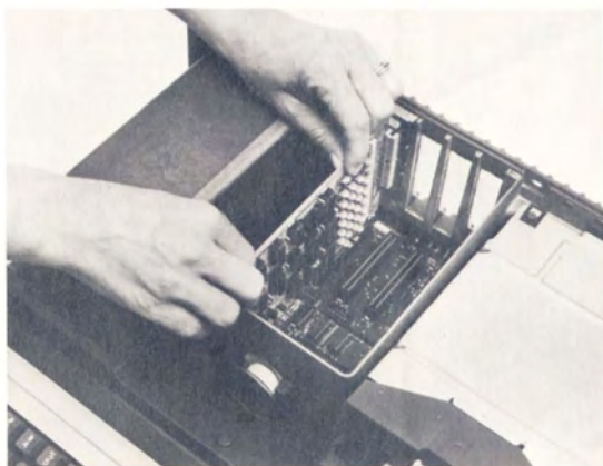
Installing a Peripheral Card
